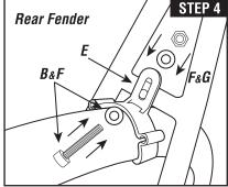
Step 4: Mounting Rear fender: Remove rear wheel. Snap the plastic clip (E) onto the rear fender and bolt it to the seat stay bridge using the 25mm bolt (B) and washer (F). Secure with lock nut (G) and washer (F). Tighten to 45 in lbs or 5.1 Nm
