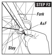
STEP F2: Your fender comes with Release Tabs that are designed to release the fender stavs from the fork if debris becomes lodged in between tire and fender. Using the 12mm bolts (A) and washers (F), bolt the Release Tab/Stay Assembly to the outside of the threaded eyelets on your fork (use lower eyelets if you have two per side). Tighten to 20 Inlbs or 2.3 Nm.
