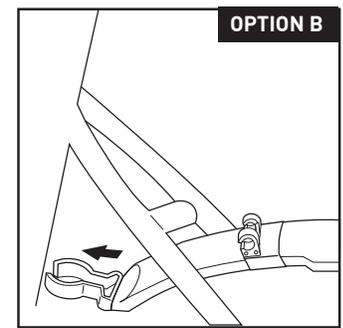
**OPTION B:** If no hole is present on the seat stay bridge, snap plastic clip (A) onto fender as shown above. Attach front of rear fender to seat tube and adjust plastic clip to line up with seat stay bridge. Secure clamps around bridge. If clamps don't fit snugly, we don't recommend using this fender.
