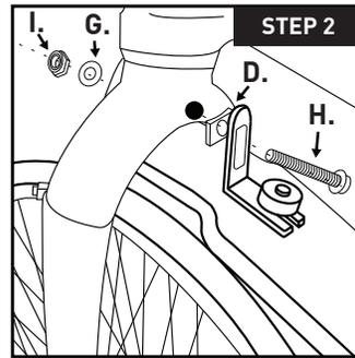
**STEP 2:** On the back side of the fork crown, thread the 43mm bolt (H) through the steel hanger and concave washer (D). Secure with lock nut (I) and washer (G).
