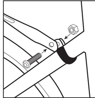
**STEP 2 CONT'D:** If bicycle frame does not have upper rack mounts, rubber coated P-clamps (E), nuts (D), and upper mounting bolts (B) can be used.
