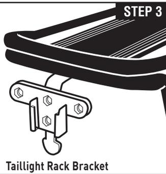
**STEP 3:** Mount the L-Bracket to rack using one bolt (A), one washer (C), and one nut (D). A standard reflector can be mounted direct to the L-bracket. A Planet Bike rear light can be mounted to the L-bracket with the addition of a Planet Bike Taillight Rack Bracket (Part# 3108, sold separately).
