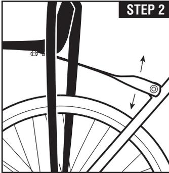
**STEP 2:** Attach the rack's upper stays to upper rack mounts using upper mounting bolts (B) and two washers (C). Position rack level with the ground. Various stay lengths can be set by removing pre-installed hardware, extending stays, and re-securing hardware. You may need to slightly bend stays into appropriate position. Tighten down all hardware (6-8 Nm / 53-69 in lbs).
