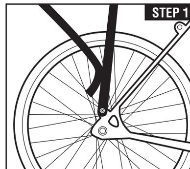
**STEP 1:** Attach rack to bike frame at the lower rack mounting points using lower mounting bolts (A) and two washers (C). Do not fully tighten bolts yet.
