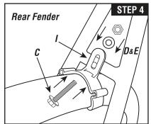
Step 4: Mounting rear fender: Remove rear wheel to install rear fender. Snap the plastic clip (I) onto the rear fender and bolt it to the seat stay bridge using the 25mm bolt (C). Secure with lock nut (E) and washer (D).
