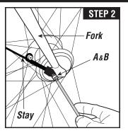
Step 2: Your fenders come with Release Tabs on the front fender that are designed to release the fender stays from the fork if debris becomes lodged in between tire and fender. Using the 12mm bolts (A) and washers (B), bolt the Stay Assembly/Adjustment Bracket to the outside of the threaded eyelets on your fork (use lower eyelets if you have two per side). Tighten to 20 lnlbs or 2.3 Nm.
