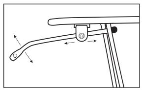
**STEP 2:** Attach the rack's upper stays to upper rack mounts on the bike using mounting bolts (A) and two washers (B). Curved stays are installed on your rack at the factory and can be positioned one of two ways. Alternate straight stays are also included and may fit better on some bikes. Position rack level with the ground. Stay lengths can be set by extending stays and securing hardware. Tighten down all hardware (6-8 Nm / 53-69 in lbs).
