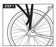
STEP 1: Attach rack to bike frame at the lower rack mounting points using mounting bolts (A) and two washers (B). Do not fully tighten bolts yet.
