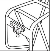
**STEP 3:** A standard reflector can be mounted direct to the mounting plate on the back of the rack. A Planet Bike rear light can be mounted to the mounting plate with the addition of a Planet Bike Taillight Rack Bracket [Part# 3108, sold separately).
