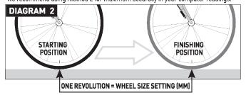
**METHOD 2:** WHEEL ROLL OUT For best results, find a flat smooth surface to perform the wheel roll out and inflate your tires to riding pressure.
