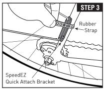
Position rear fender as shown in Fender Location Diagram on previous page. Attach the SpeedEZ Quick Attach Brackets to the seat stays by wrapping rubber straps around the seat stays and looping over bracket hooks. Be sure to pull firmly on straps for a secure fit. Note: For excess portion of rubber straps, either A) Double over and loop onto outside hooks or B) Cut off excess making sure to leave enough strap for future removal and installation.
