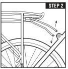
STEP 2: Mount upper stays on rack to upper mounts on bike using two Bolts (D) and two Washers (B). If bicycle frame does not have upper rack mounts, Mounting Brackets (E), Nuts (F), and two Washers (B) can be used as upper attachment points on the seat stays.
