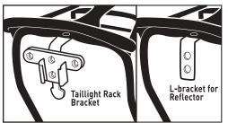
STEP 4: Mount reflector or rear light [not included] to Rear Reflector/Light Mount. A standard reflector can be mounted direct to the L-bracket. A Planet Bike rear light can be mounted to the L-bracket with the addition of a Planet Bike Taillight Rack Bracket (Part# 3108, sold separately).
