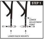
STEP 1: Mount rack to bike using two Lower Mounting Bolts (A), Washer (B) and two Mounting Spacers (C) to secure lower rack mounts of rack to lower mounts on bike. Do not fully tighten bolts yet.
