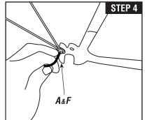
STEP 4: Mounting rear fender: Remove rear wheel to install rear fender. Using two 12mm bolts (A) and two washers (F), bolt the fender stay to the outside of the threaded eyelets on the frame. Tighten to 35 lnlbs or 4 Nm.
