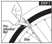
**STEP 7:** Rear fender adjustment: Loosen the 10mm nuts that attach the stays to the rear fender and position the fender so that it conforms to the curvature of the tire without rubbing. Make sure you have a minimum of 10 mm of clearance between the tire and fender. Tighten the nuts snugly, but don't use all of your strength or you risk breaking the hardware. Tighten to 30 Inlbs or 3.4 Nm.
