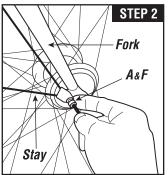
**STEP 2:** Your fenders come with Release Tabs on the front fender that are designed to release the fender stays from the fork if debris becomes lodged in between tire and fender. Using the 12mm bolts (A) and washers (F), bolt the Release tab/Stay Assembly to the outside of the threaded eyelets on your fork (use lower eyelets if you have two per side). Tighten to 20 Inlbs or 2.3 Nm.
