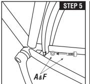
**STEP 5:** Attach front end of fender to chain stay bridge using bolt (A) and washer (F). If no chain stay bridge hole is present, fasten fender to the bridge with a zip tie (I). If no chain stay bridge is present, we do not recommend using these fenders.
