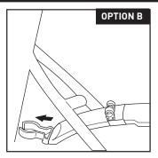
OPTION B: If no hole is present on the seat stay bridge, snap plastic clip [A] onto fender as shown above. Attach front of rear fender to seat tube and adjust plastic clip to line up with seat stay bridge. Secure clamps around bridge. If clamps don't fit snugly, we don't recommend using this fender.
