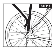
STEP 1: Attach rack to bike frame at the lower rack mounting points using lower mounting bolts (A) and two washers (C). Do not fully tighten bolts yet.
