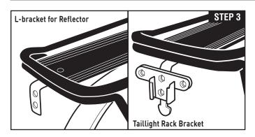
**STEP 3:** Mount the L-Bracket to rack using one bolt (A), one washer (C), and one nut (D). A standard reflector can be mounted direct to the L-bracket. A Planet Bike rear light can be mounted to the L-bracket with the addition of a Planet Bike Taillight Rack Bracket (Part# 3108, sold separately).
