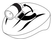
**STRAP FITS OVER LIGHT** La bande se fixe sur la phare **STEP 1:** Attach the light to the mount and set it on the appropriate part of the helmet.
