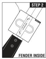
STEP 2: Cut out square template below and mark holes to be drilled on inside surface of fender. Bracket placement should be just above themud flap on the rear fender only. Be sure to align center line on template with center of fender to ensure the light is positioned straight.
